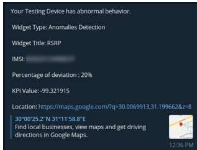
Above left INOS report of RSRP in LTE, identifying an anomaly with 20% deviation Above right Telegram Notification for a customer with certain Anomaly Detection
